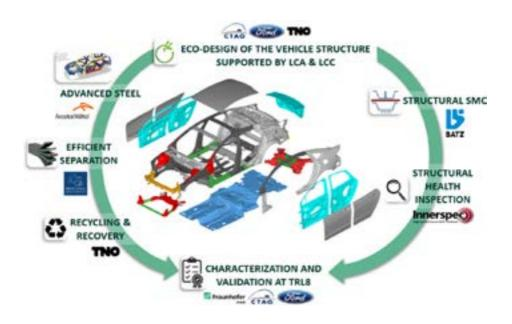
The body-in-white (BiW) of ALMA's concept car is **160 kg lighter**, representing a **22% weight reduction** compared to the baseline BEV BiW. Over the car's entire service life, the use of other materials and weight reduction contributes to a total reduction of **1850 kg CO2-eq**, a **24% decrease** in emissions.
