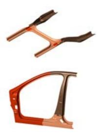
Fraunhofer ITWM demonstrated that their simulation methods make it possible to experiment with many material models, minimising the need for experimental calibration, thereby saving precious time and resources. In collaboration with Ford, BATZ and CTAG, Fraunhofer demonstrated that the SMC components, developed by BATZ, meet crash safety requirements, significantly reducing vehicle weight.
